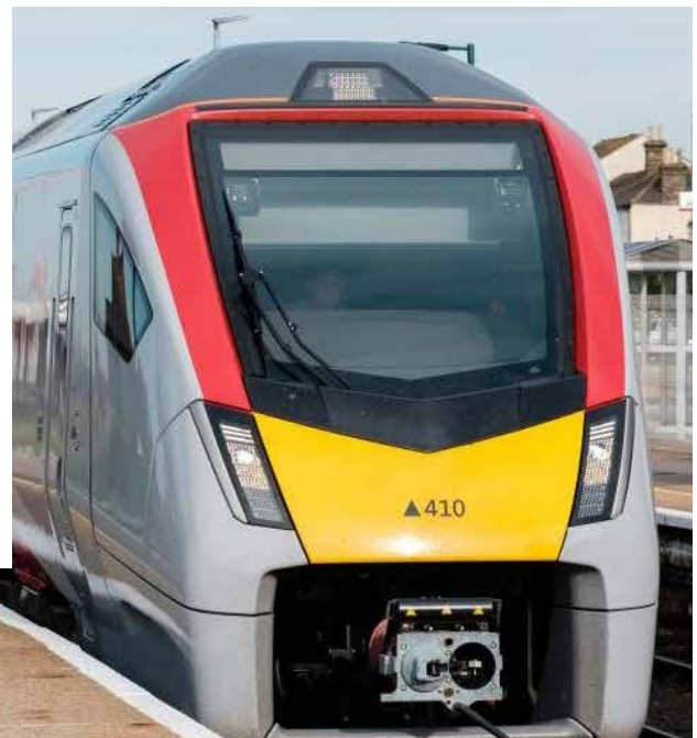
One of 38 new bi-mode trains entering service on the Greater Anglian network. Built by Stadler in Switzerland, they offer state-of-the-art, environmentally friendly technology and feature low floor and level boarding, vastly improving the customer experience.
